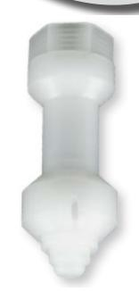
The HydroWhirl® Mini PVDF tank cleaning nozzle directs the cleaning water through a rotating head at the tip of the spray assembly and produces a vigorous moving spray action against all areas of the tank wall.
